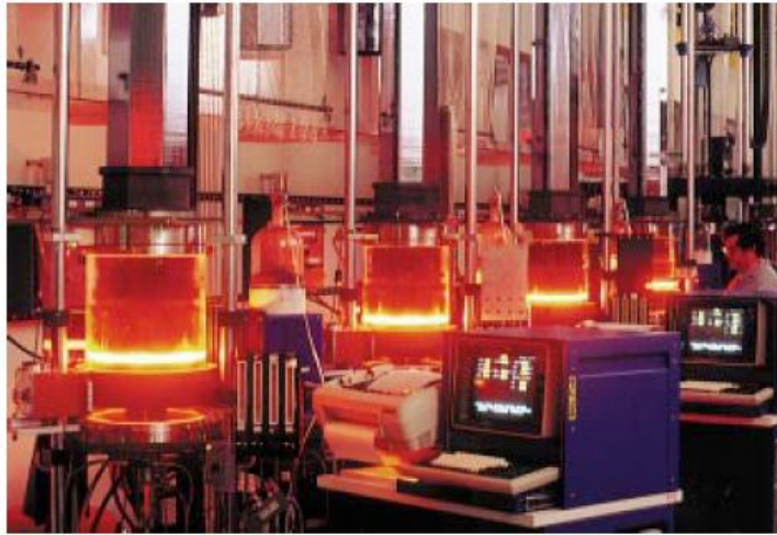
ASE Americas' production line for EFG crystal growth.
